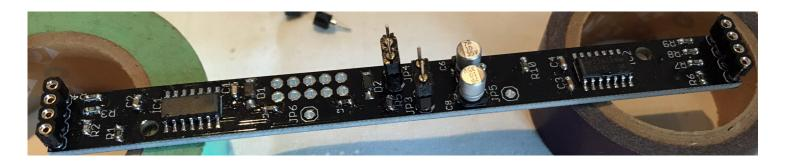
6.Place the x2 pines and the top pcb to solder both sides.
