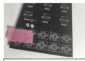
1. Put some tape on the front side of the pcb.
