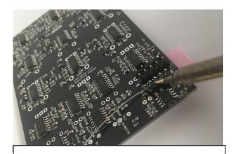
2. Insert the male header pins with the longest part upside down and solder.
