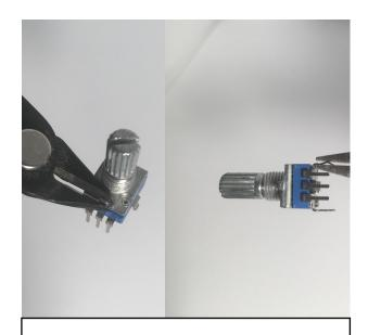
4. Remove the anti-rotation tag, straighten up the bracket.
