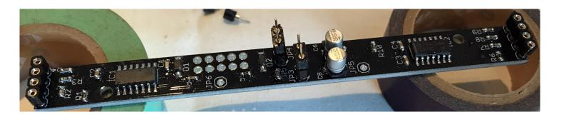
6. Place the x2 pines with the top pcb to solder both sides.
