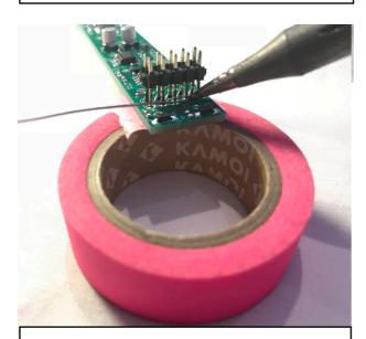
3. Solder the pins from the top side as in the picture .
