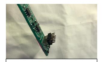
2. Insert the male header pins with the longest part upside down.
