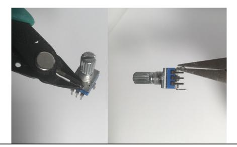
1. Remove the anti-rotation tag, straighten up the bracket.
