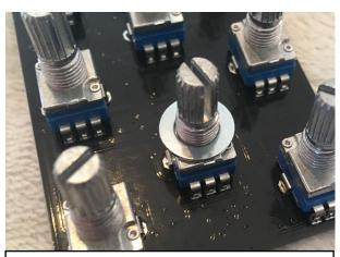
5.Place potentiometers and jacks on the board but don't solder them. Put 2 washers per pot, place the front panel and screw it.
