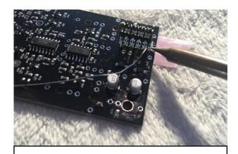
2. Insert the male header pins with the longest part upside down and solder.
