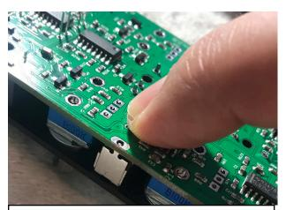
5.Press down the sliding switch, solder 1 pin and make sure is centered. Finish soldering the mounting hardware
