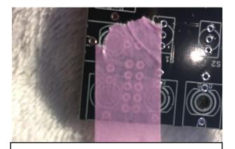
1. Put some tape on front side of the pcb.
