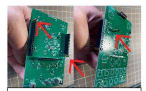
5. Screw the couple of bigger metal spacers at the back of the control board and the small one in the front side like the picture is showing.
