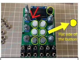
8. Place the hardware, screw the oled to the metal spacer and place 2 washers per pot ( double check again POLARITY but DON'T SOLDER YET )
