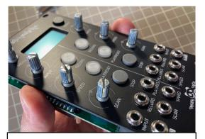
10. Pull up the pots and screw them to the panel, don't pull up the encoder.Be careful if the panel is not correctly placed pots or buttons can fall out.
