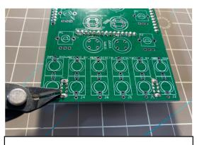
4. Carefully cut the pins so the jacks can settle properly.
