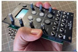
9. Carefully place the panel and press it otherwise the buttons or pots can easily fall out. Check all jacks are correctly aligned after this step screw the jacks to the panel.
