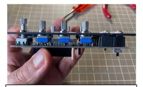
11. Check the panel, pots and jacks are correctly balanced before soldering. Don't pull up the encoder like the pots.
