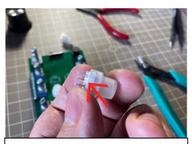
7. Check the LED colour marked on the push button, check polarity make sure the flat side of the button matches the flat side of the silkscreen.
