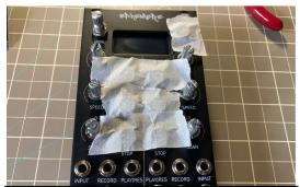
12. Put tape on the buttons to continue with the soldering session. Do not apply too much time and heat soldering the middle legs of the buttons, BEWARE LED'S CAN BE DAMAGED.
