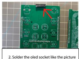
2. Solder the oled socket like the picture is showing.
