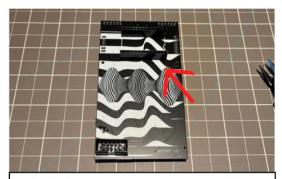
Solder the power connector and the female sockets for the mini-PCB as showing in the pic, you can use the mini-PCB to align it better.
