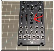
9. Place the sliding switches. The 3 position switch (the red one) must be inserted where the arrow is showing. With all hardware aligned, screw the panel. Now continue to solder.
