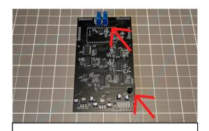
1. Solder both trimmers and the -5V regultator.
