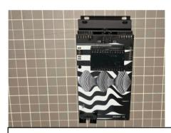
11. The trimmer on the right will calibrate C1 and the trimmer on the left C9. Continue with calibration.
