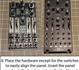
8. Place the hardware except for the switches to easily align the panel. Insert the panel to check the hardware is perfectly aligned. Remove the panel to place the switches, this way will be easier.
