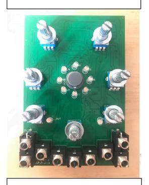
3. Place jacks, pots, 2 washers per pot and THE GRAY BUTTON MUST BE POSITIONED WITH THE FLAT SIDE TO THE LEFT.
