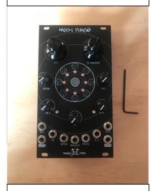
4. Insert the knobs and tide the big ones with the allen key.
