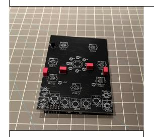
1. Solder the power connector, the 330pF caps and LM337 IC if the SMD from the back is not soldered.
