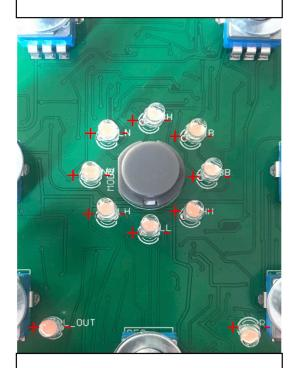
4. IMPORTANT BE CAREFUL WITH THE POLARITY OF THE LEDS. THE LONG LEG GOES TO THE POSITIVE.
