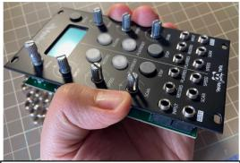
Carefully place the panel and press it otherwise the buttons or pots can easily fall out. Check all jacks are correctly aligned after this step screw the jacks to the panel.
