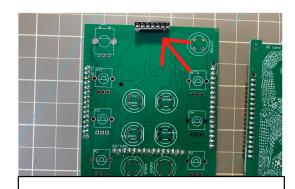
2. Solder the oled socket like the picture is showing.
