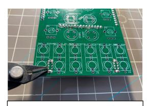
4. Carefully cut the pins so the jacks can settle properly.
