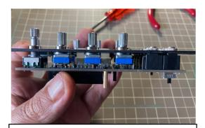
11. Check the panel, pots and jacks are correctly balanced before soldering.
