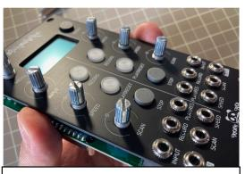
10. Pull up the pots and screw them to the panel, don't pull up the encoder. Be careful if the panel is not correctly placed pots or buttons can fall out.
