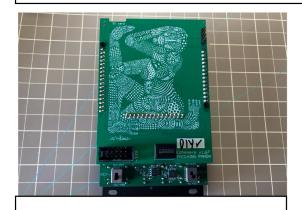
13. Attach and screw the back of the PCBA, place the knobs.
