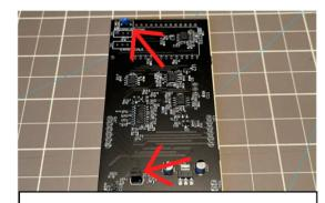
2. Solder the **3.9nF** cap and the -5V regulator as shown.
