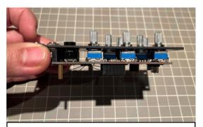
7. Pull the LED's to the bottom, align the panel with the hardware, check the pots are pulled up, continue with the soldering.
