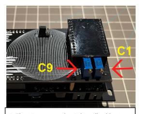
9. The trimmer on the right will calibrate C1 and the trimmer on the left C9. Continue with calibration.
