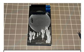
Beware! Solder the trimmers and the female sockets for the mini-PCB at the back of the main PCB. The SILKSCREEN of those components is incorrect.
