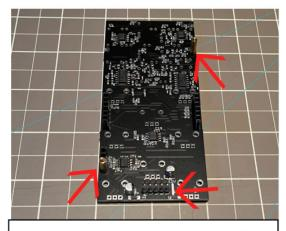
3. Screw the metal spacers and solder the power male connector.
