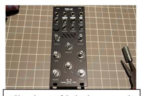
6. Place the rest of the hardware, screw the panel, DO NOT SOLDER YET.
