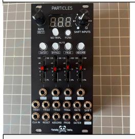
10. Attach both PCB's, place the knobs and power the module. The MAIN PCB has been fully tested.
