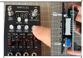
8. Make sure all buttons can be pressed, otherwise align better the panel with the PCB, the buttons needs some room to bounce.
