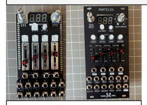
7. Place the segment display, attach the panel, screw all nuts but DO NOT SOLDER YET.
