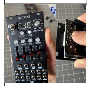
9. Carfully bring the segment display to the front, try not to rubber it to the panel, it can easily be scratched, when you think is proprely centered, solder 1 pin and make sure it is to solder the rest of the pins. Continue to solder the rest of the hardware.
