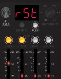
Pressing and holding the FUNC button while simultaneously pressing the encoder directs you to the RESET PULSES menu. With the Channels buttons activated, trigger inputs possess the capability to interrupt (choke) the repetition pulses of other Channels if their respective buttons are also activated
