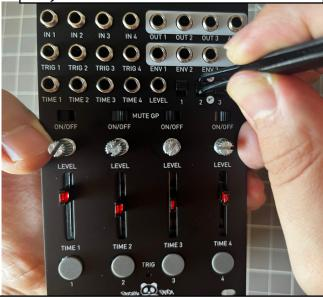
9. Remove the panel, insert the 8 sliding switches, when placing the panel back try to bring up the switches with your hand from the bottom, when the switches are up you can screw a few nuts to prevent them to fall out.
