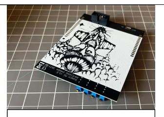
2. Solder the power connector and the 4 multiturn trimmers.
