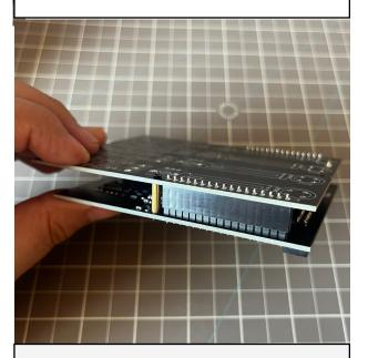
4. Attach both PCB's with female/male connectors and metal spacers, then solder them.
