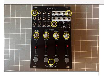
7. Place the panel, screw 3 jacks nuts, 4 pot nuts, the small screw, all circled in yellow.
