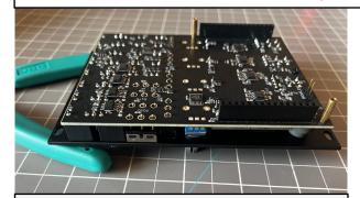
10. With the help of the side cutters place the module upside down horizontally **only** solder the middle pin from the switches, then make sure they can slide correctly before proceeding to solder the rest of the pins.
